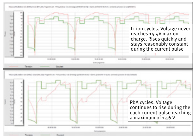
Fig 10: December cycle tests for lithium-ion and lead-acid batteries
