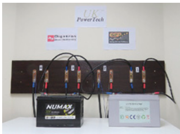
Fig 1: As received Numax lead-acid and Chinese lithium-ion batteries
