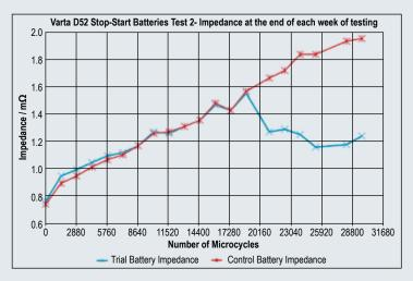
sulfate", subject to Ostwald ripening, is very hard to dissolve. Clearly, if our charging protocol had been used from the beginning of the test, as it would on a real car, the battery would never have a buildup in impedance at all. It would then have a better performance and, quite possibly, twice the life. Not bad for a bit of software, huh?
