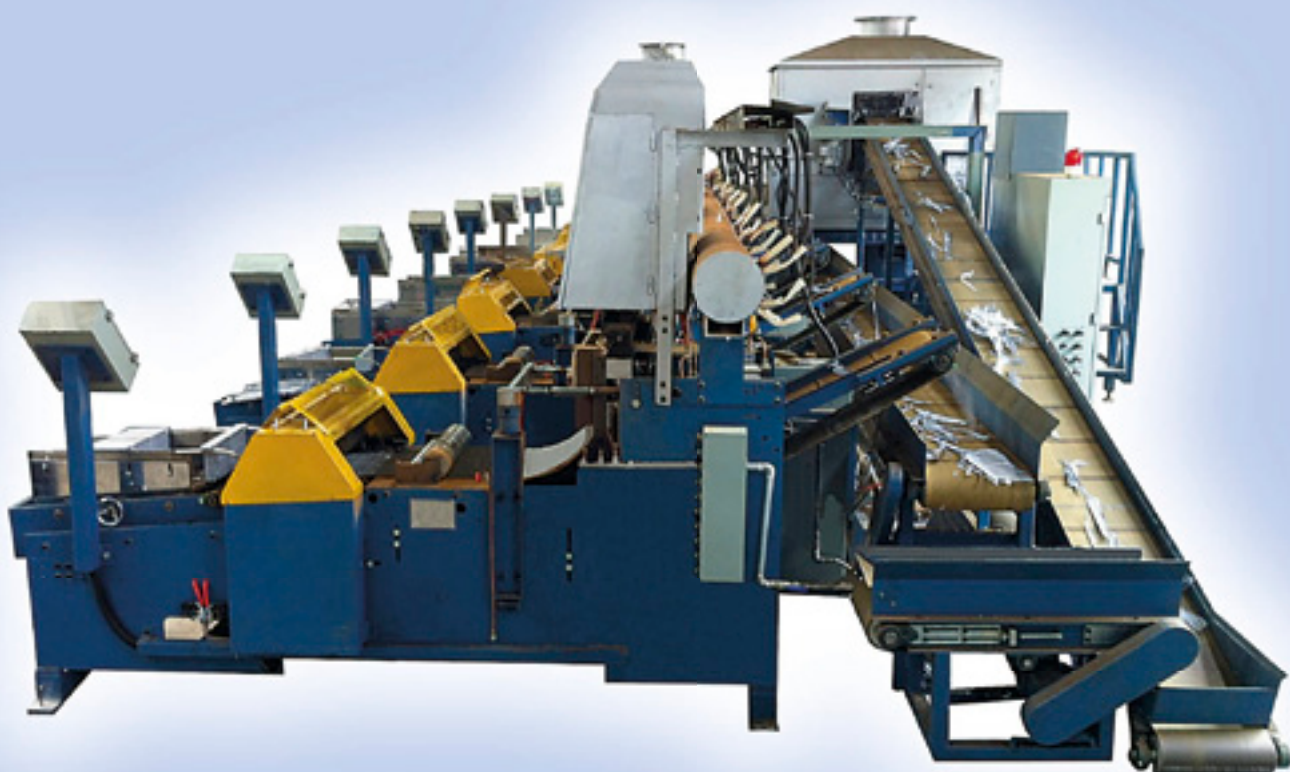
Centralized lead supply system — one lead pot with several casting machines
