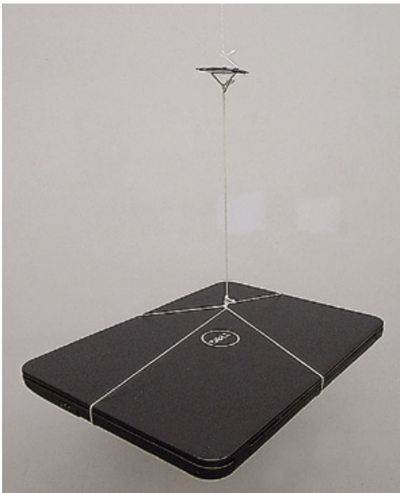
Laptop suspended from a thin structural supercapacitor Source: Vanderbilt University
