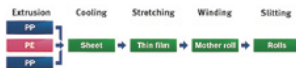
Figure 2. Processing schematic of a trilayer separator, with lamination between the extrusion and cooling steps (from Mitsubishi Plastics).
