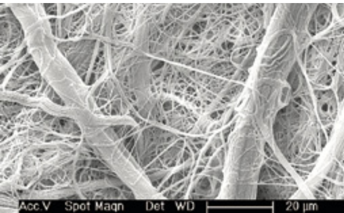
Figure 10. SEM image of Dreamweaver separator, highlighting the combination of nano and microfibers that provides tight pore size control.
