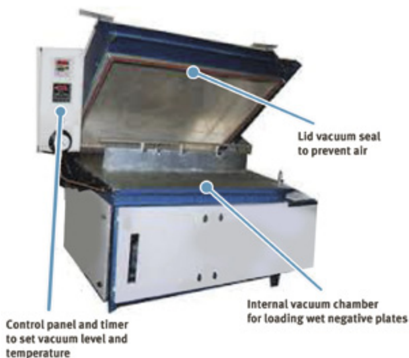
Figure 5 Example of simple negative vacuum dry charge chamber
