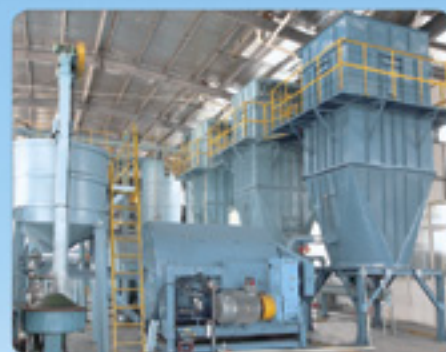
Plate Making Equipments (Lead Oxide Ball Mill)
