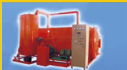
Vacuum Drying Oven for both negative plate and positive plate
