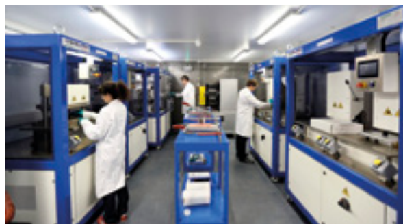
The dry room has less than 1% relative humidity.
