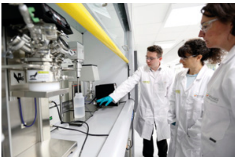
Project engineer Philip Hallam describes the small-scale electrode slurry mixing equipment to research fellows Stefania Ferrari and Melanie Loveridge.
