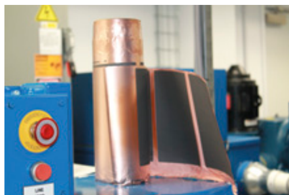
Calendring compacts the coating to improve the energy density of the battery electrodes.
